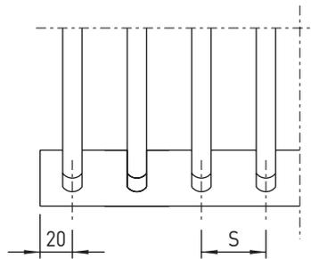
Element spacing  $S = 40 \text{ or } 60 \text{ mm}$
