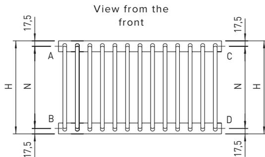
Centre distance N is calculated as: Radiator height (H)-35 mm
