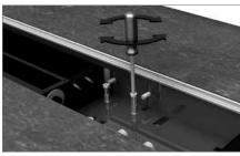
Double height adjustment by means of the anchoring on the outer casing and by fine adjustment with the bolts in the inner housing (adjustable from 6.2 to 8 cm).
